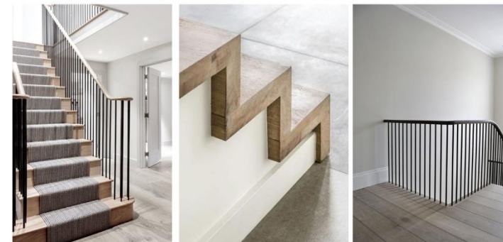
Stair Case Timber treads and risers with dark railings and timber handrail. Overhang detail to edges would be a nice touch if wanted (centre top image) Central runner added for comfort and aesthetics – design TBC
